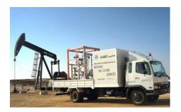
Haimo's **Low Production Tester**–LPT is developed primarily to address accurate measurement of low flowing and slugging wells.
